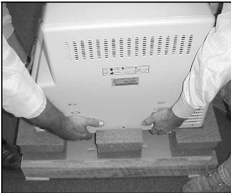
Figure 9. Two People Placing the Scanner onto the Skid
