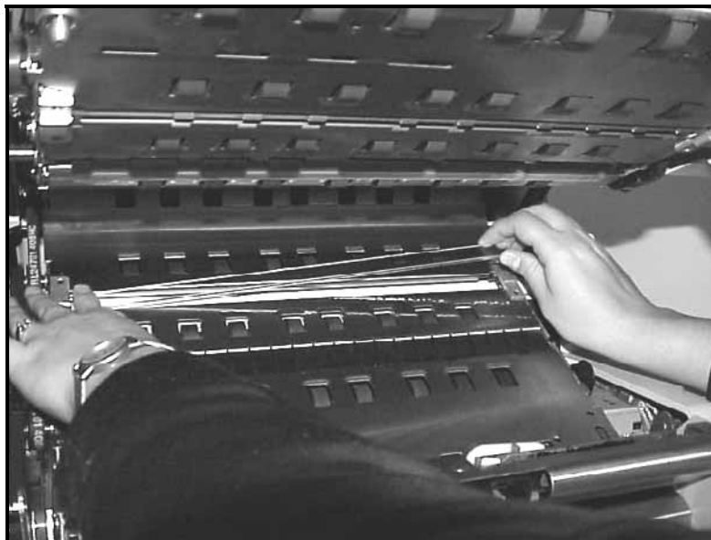
Figure 38. Replacing the Glass Flat
