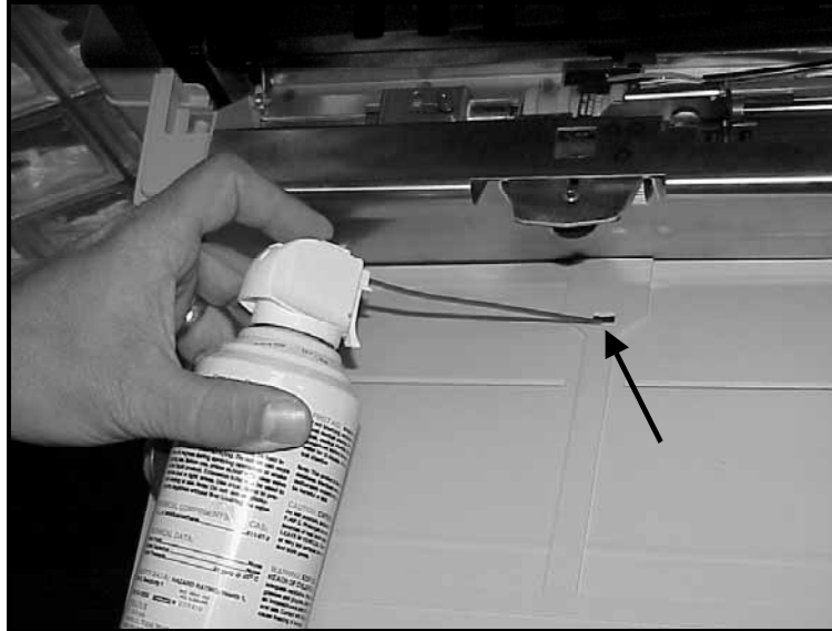
Figure 44. Feeder Sensor Location
